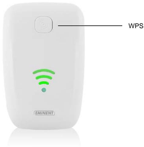
6. The connection between your wireless router and the EM4595 wireless repeater will be established automatically (this will take approx. 1 minute including reboot). The smart led indicator will stop flashing and indicate the signal strength. Wait until the WiFi led turns blue.
