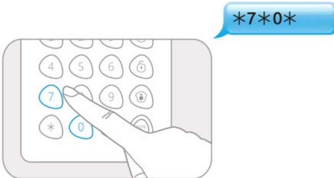
When one beep is heard and the LED indicator keeps on for 10 seconds, the setup is successful.
