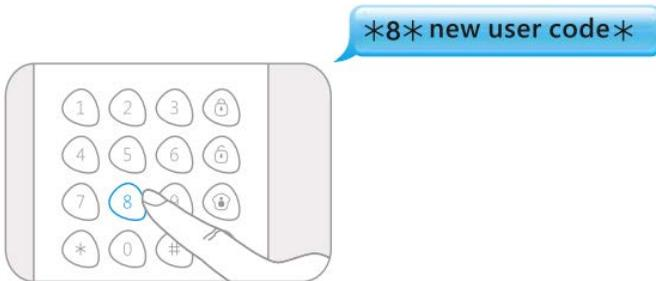
When one beep is heard and the LED indicator keeps on for 10 seconds, the setup is successful.
