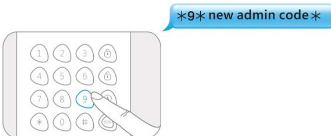
When one beep is heard and the LED indicator keeps on for 10 seconds, the setup is successful.
