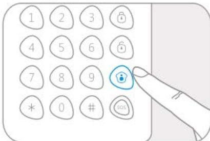
When the alarm panel receives the signal, the siren will beep once and the Home Mode indicator will light, the alarm system enters Home Mode state.
