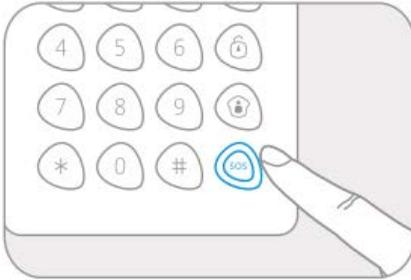
When the control panel is not in SOS Speed Dial mode, user needs to input user code or admin code before holding the [SOS] key for 3 seconds to send an alarm.
