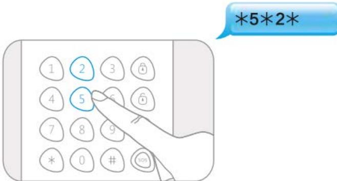
When one beep is heard and the LED indicator keeps on for 10 seconds, the setup is successful.
